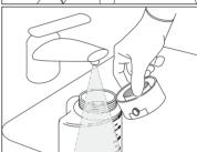
Remove any detergent remaining with a soft cloth with low fiber-release dampened with sterile water in order to maintain the disinfection;
