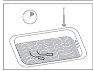
Remove the insert from the ultrasonic tank and rinse with distilled water;
