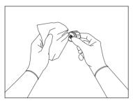
Dry the inserts torque wrench using a soft cloth with low fibre release
