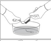
During immersion in the enzymatic solution, delicately brush the surface of the insert using the brush with soft nylon bristles to eliminate all traces of visible dirt. Thoroughly clean the difficult areas such as sharp edges;
