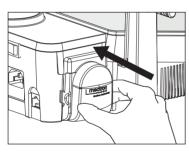
Re-position the plastic cover on the peristaltic pump.
