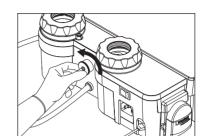
Extract the filter and wash it under running water to eliminate the impurities that obstruct it.
