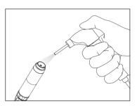
① CAUTION: Before starting the sterilization cycle, make sure that the insert is thoroughly dry both internally and externally. To do this, blow compressed air both externally and through the internal passage hole. This will prevent the appearance of stains, streaks on the surface or oxidation inside the insert.
