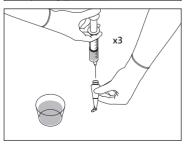
Using a syringe, inject the enzymatic detergent solution three times inside the cavity of the polisher tip to effectively remove the residues from the internal surface;
