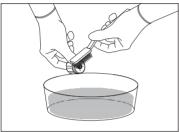
During immersion in the enzymatic solution, delicately brush the surface of the wrench using the brush with soft nylon bristles to eliminate all traces of visible dirt both in the internal and external part;
