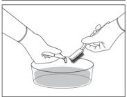
During immersion in the enzymatic solution, delicately brush the surface of the polisher tip using the brush with soft nylon bristles to eliminate all traces of visible dirt. Thoroughly clean the difficult areas such as edges and, in particular, the gaps;
