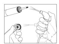
**(i) CAUTION:** The scaler handpiece electric contacts must be dry before the end of the sterilization cycle, before connection of the device lead. Always make sure that the connector electric contacts are entirely dry; dry them by blowing compressed air if necessary.
