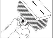
Completely rinse with tap water to eliminate any detergent residues and perform the last rinse with distilled water;
