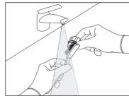
Delicately brush the surface of the wrench with a brush with soft nylon bristles using distilled water;
