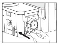
4 Connect the new peristaltic pump to its seat until a "click" sound is heard and then connect the two pump tubings to their respective couplings positioned beneath the pump;
