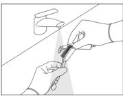
Delicately brush the surface of the polisher tip under running water using the brush with soft nylon bristles;
