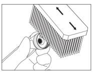
Accurately rinse with tap water to eliminate any detergent residues and perform the last rinse with distilled water;
