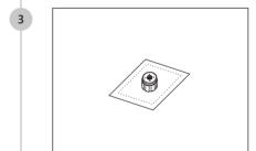
Seal the K9 wrench individually inside a disposable bag for sterilization.
