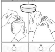
Once you've finished the cleaning procedure, check the irrigation solution container and the cap under an adequate source of light, paying attention to the areas that could conceal dirt residues (cavities, grooves) and, if need be, repeat the cleaning cycle.
