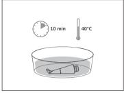
24 Let the polisher tip soak for 10 minutes at 40°C ±2°C. This procedure reduces the amount of blood, protein and mucous present on the polisher tip;
