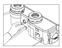
Re-introduce the filter into its seat and screw the knurled bush back into its housing tightly until it is fully in position.
