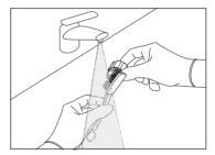
Using a 20 ml disposable syringe, flush the surface of the wrench 3 times with 20 ml of enzymatic detergent solution;
