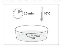
6 Let the insert soak for 10 minutes at 40°C ±2°C. This procedure reduces the amount of blood, protein and mucous present on the insert;
