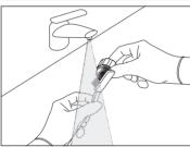
Delicately brush the surface of the wrench with a brush with soft nylon bristles under running water;
