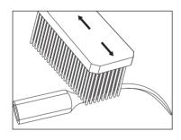
Delicately brush the surface of the insert under running water (drinking water, temperature 20°C+/- 2°C), in particular the parts that are difficult to access (cavities, structured surfaces, etc.) using a brush with soft nylon bristles;
