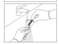
Rinse the internal canal of the insert with distilled water injected under pressure (3.8 bar) for at least 10 seconds to eliminate all residues;
