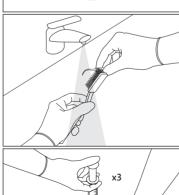
8 Delicately brush the surface of the insert under running water using the brush with soft nylon bristles;
