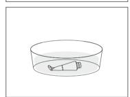
Delicately brush the surface of the polisher tip again using the brush with soft nylon bristles:
