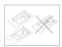
Seal the wrench individually inside a disposable bag for sterilization.
