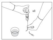
9 Using a 20 ml disposable syringe, inject 20 ml of cold demineralised water 3 times inside the cavity of the insert;
