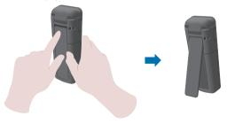
To close the stand, press the lower end of the stand to the original position.
