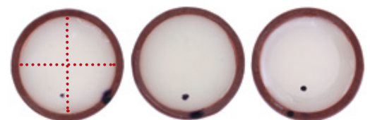
Width of cure samples in 20 mm molds. Hardness was measured at 1 mm intervals in the pattern shown. The area visibly affected by the light was always much larger than the actual cured material.
