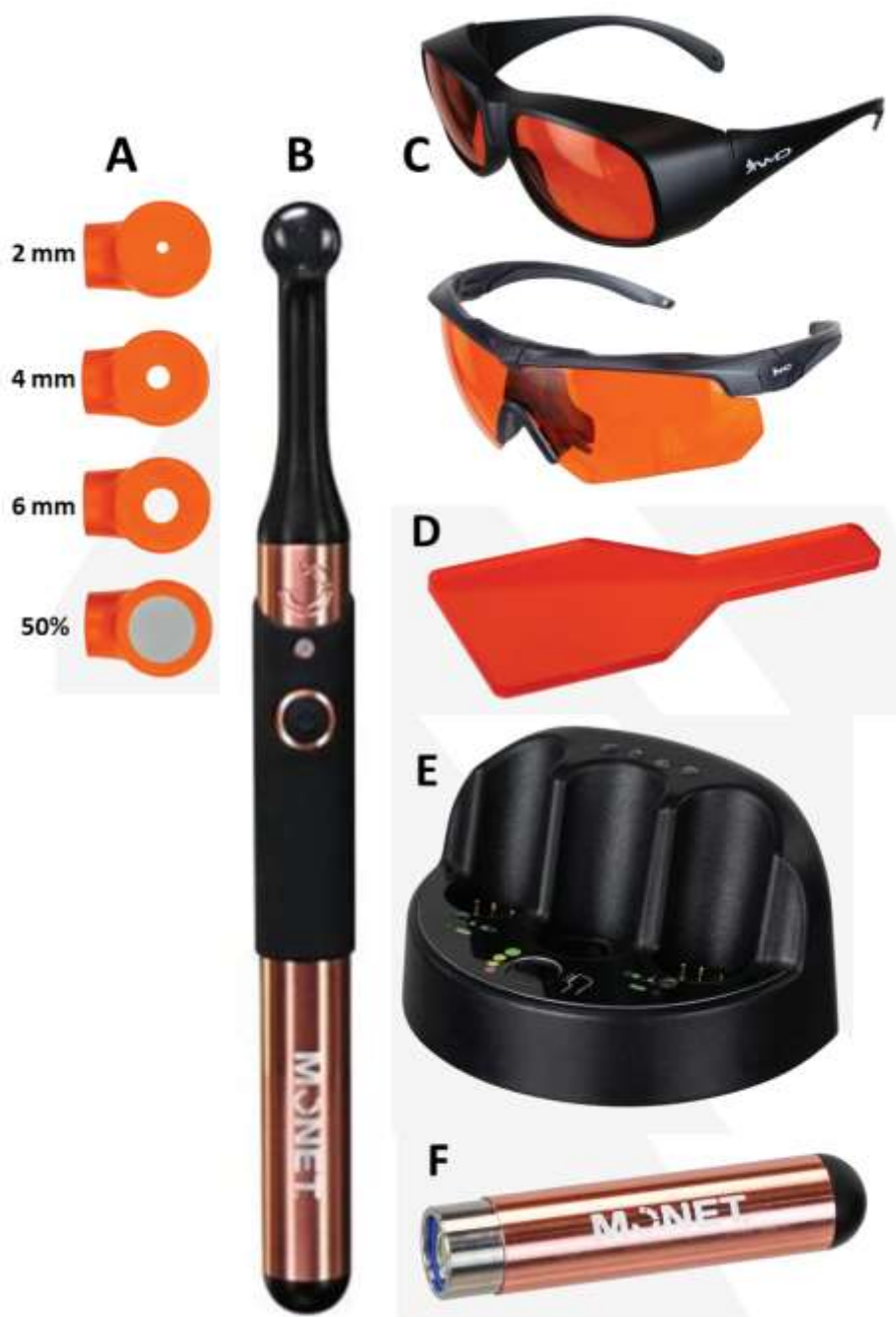
Fig. 3. The major components of the Monet™ diode laser dental curing system. The main laser unit with its rechargeable battery attached is shown in panel B. A single pushbutton operates the laser. A set of 3 beam width reducing apertures and the 50% neutral density filter are shown in panel A. Laser protective eyewear is shown in panel C, and the laser protective handheld paddle shield in panel D. The replaceable battery is shown in panel F, and the battery charging base and stand for the laser in panel E. The base also contains a power meter to check for the proper operation of the laser.
