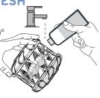
Rinse the HyGenie under gently runningwater, rotating the handles in opposite directions, until all DentalFresh foam is rinsed away and water runs clear through the device.
