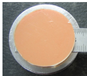
xantasil shrinkage behaviour after several weeks.
