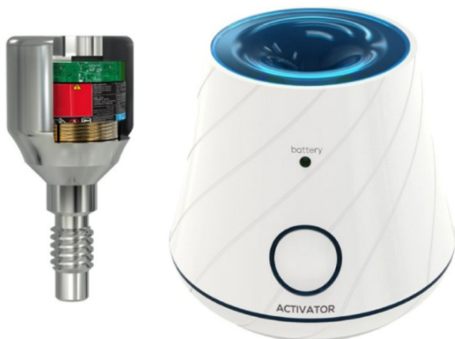
FIGURE 2 A cross-sectional view of the miniaturized electromagnetic device (MED) healing abutment (left); An activator device which triggers the battery in the MED (right).
