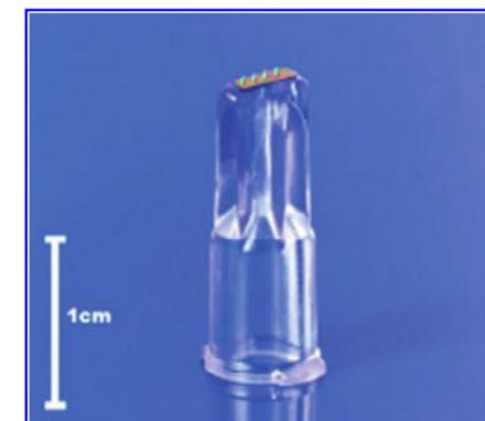
**FIG. 2.** The experimental MicronJet needle device.
